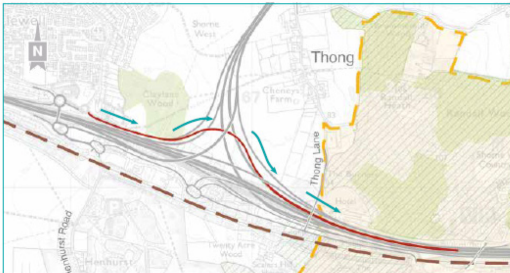
Figure 5-10. Gravesend East/Valley Drive Roundabout to M2 eastbound. A new connection has been added to the Gravesend East junction to provide a direct connection between the Valley Drive roundabout and M2 in the eastbound direction.
