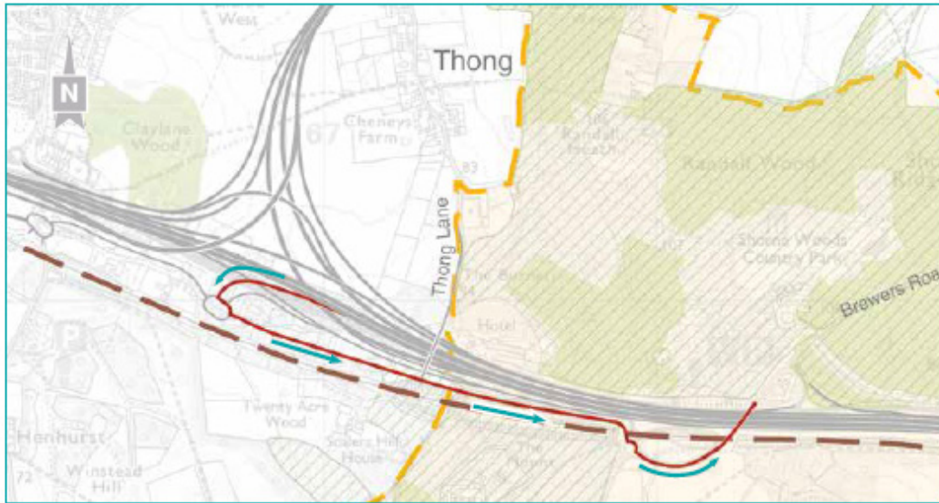
Figure 5-9. M2 westbound to Brewers Road. Leave the M2 westbound using a slip road that connects with the local network via a new roundabout at the site of the existing A2 service station. From the roundabout head east along the new two-way local link road towards the roundabout on Halfpence Lane and Brewers Road.
