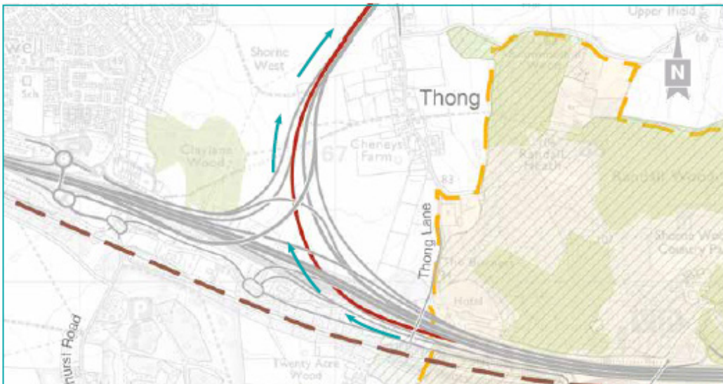
Figure 5-4. Joining the LTC from the M2/A2 westbound. Leave the M2 westbound at the exit for the LTC northbound, follow the road passing an entry slip where traffic joins from the A2 westbound parallel link road, through an underpass beneath the M2/A2, past a second entry slip road where traffic joins from the A2 eastbound and past a third entry slip road where traffic joins from Gravesend East.
