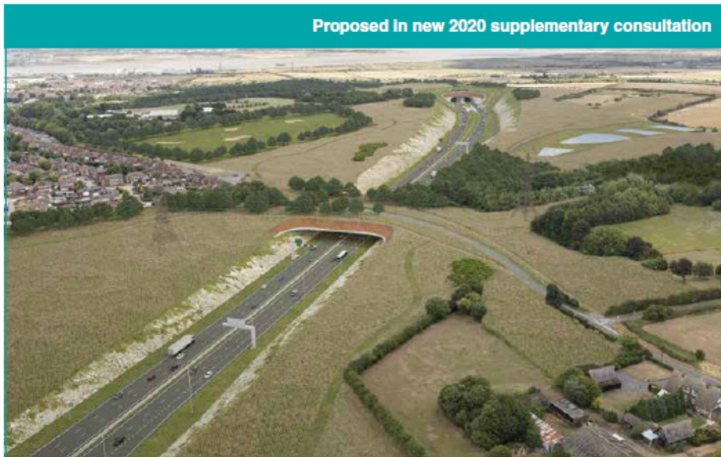
Figure 5-23. Supplementary consultation – proposed Thong Lane bridge linking Gravesend and Thong, and the approach to the south tunnel entrance, looking north
